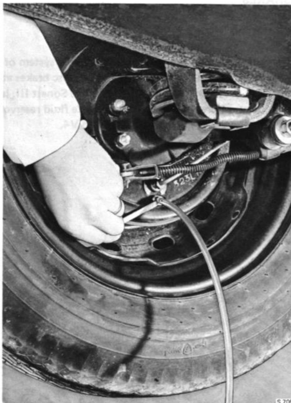
LOCATION OF BLEEDING NIPPLES, REAR END
