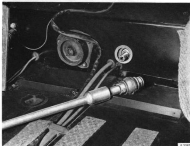
OPENING UP THE GEAR SHIFT ROD
