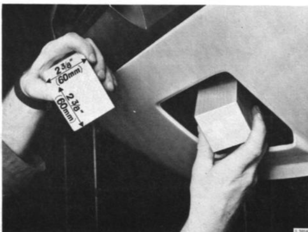
BLOCKS INSERTED BETWEEN HOOD AND RADIATOR FRAME
