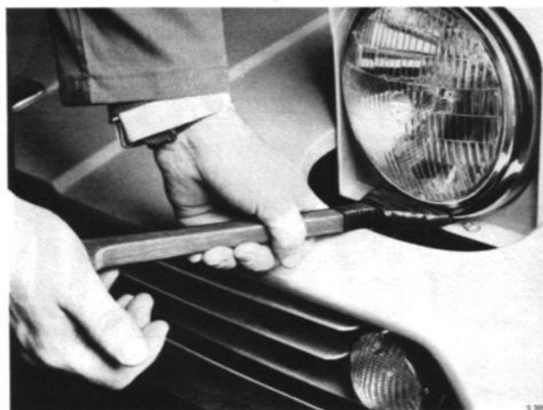
INSTALLING THE HEADLIGHT INSERT
