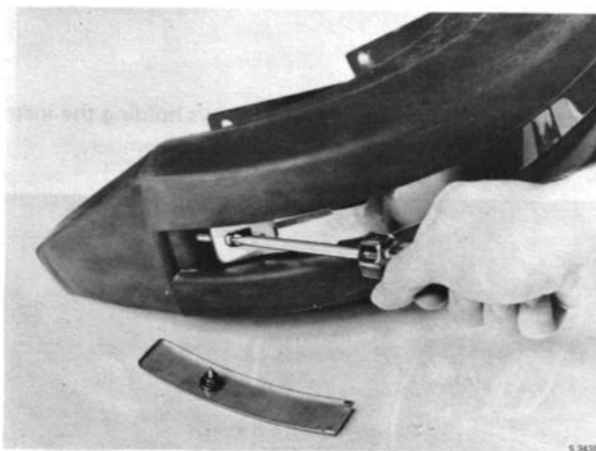
MOUNTING THE BRACING STRIP
