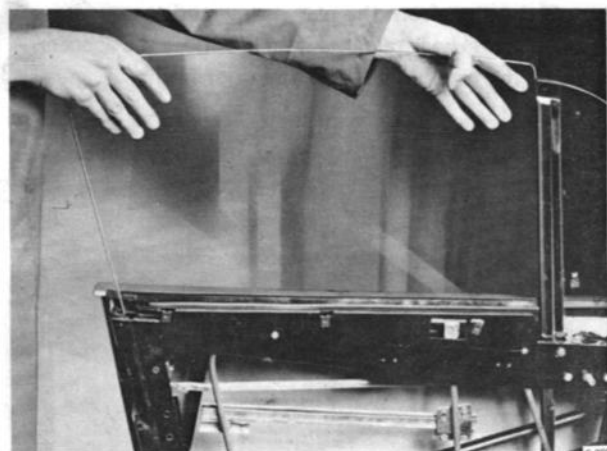
REMOVAL OF DOOR-WINDOW GLASS
