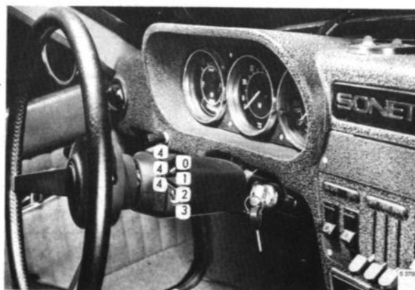
WINDSHIELD WIPER/WASHER CONTROL LEVER, AS FROM MODEL 1971
