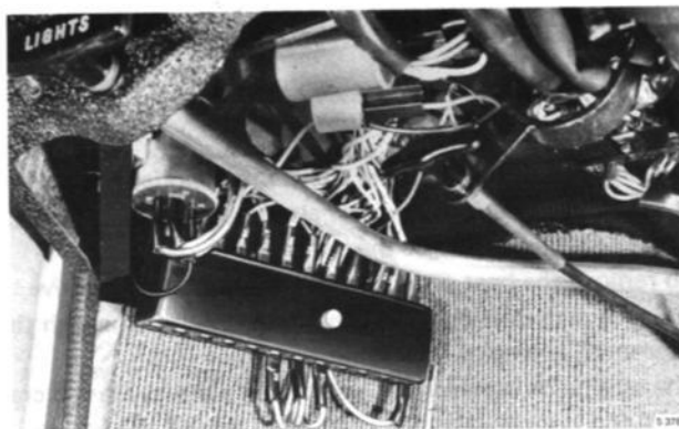
FUSE BOX UNDER INSTRUMENT PANEL
