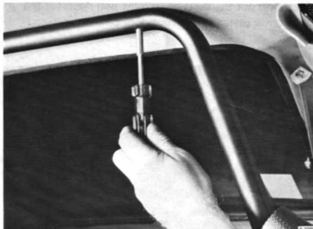
REMOVAL OF SCREWS FOR REAR WINDOW
