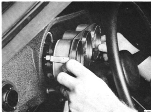
REMOVAL OF INSTRUMENT INSERT
