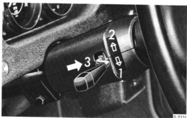
COMBINED DIRECTION INDICATOR LEVER AND HEADLIGHT DIMMER SWITCH
