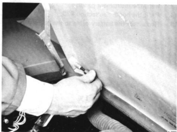
REMOVAL OF ENGINE LID
