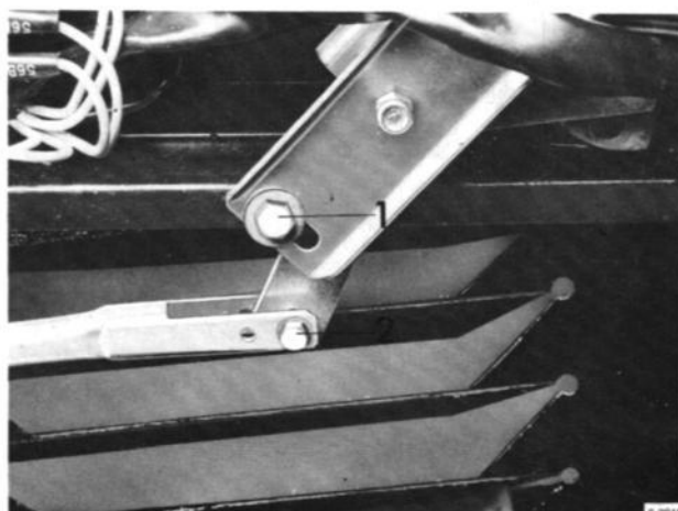
SCREWS, HEADLIGHT CONTROL
