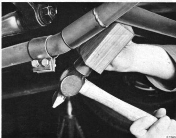
SEPARATING THE EXHAUST SYSTEMS
