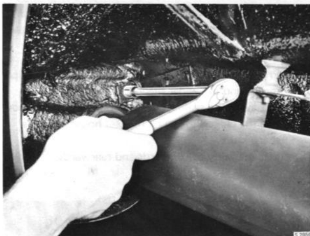
REMOVAL OF NUTS ABOVE THE REAR SILENCER
