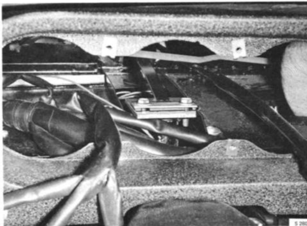
COLUMN STAND RETAINING SCREWS
