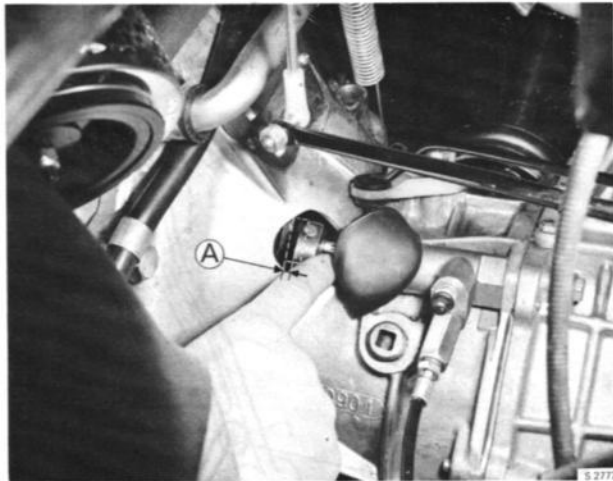
ADJUSTING THE CLUTCH CLEARANCE A = 0.16" (4 mm)
