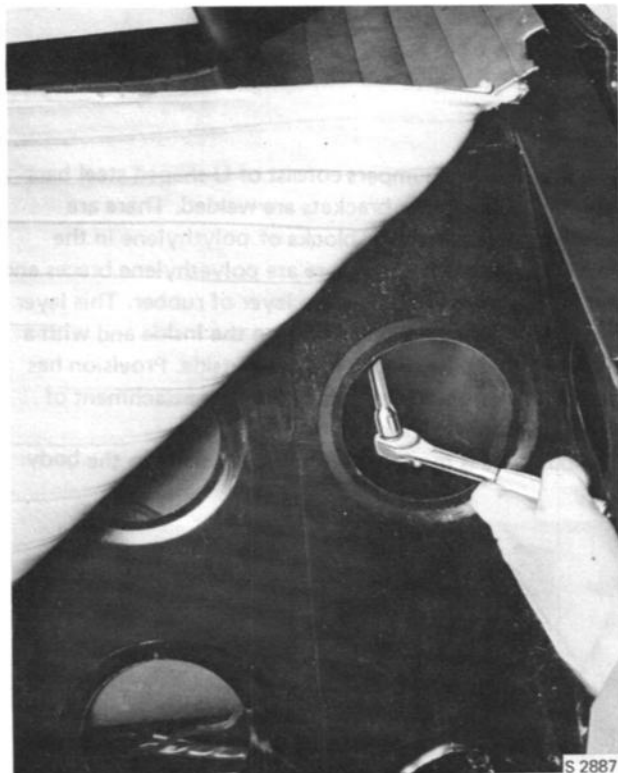
REMOVAL OF ROLL-OVER BAR RETAINING SCREWS
