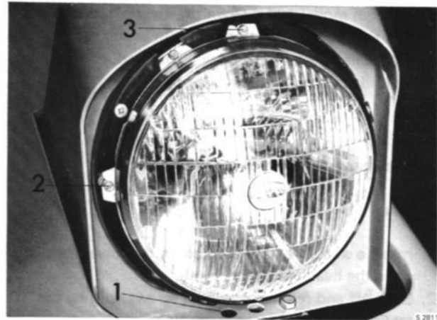
SCREWS FOR HEADLIGHT ADJUSTMENT
