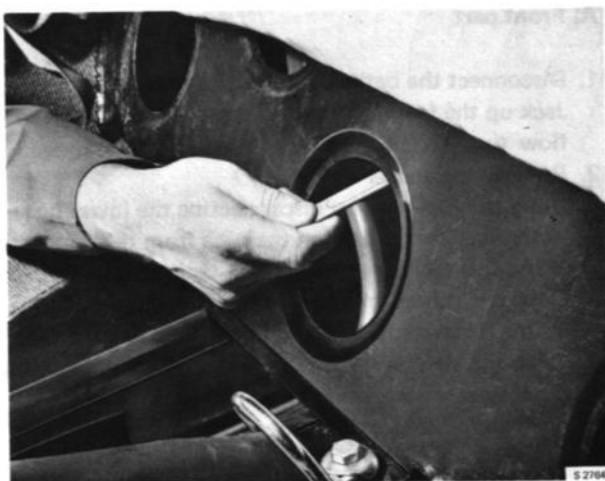
REMOVAL OF FUEL PIPE FROM TANK
