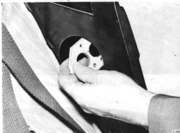
FITTING THE STRIKER PLATE AND RETAINING PLATE
