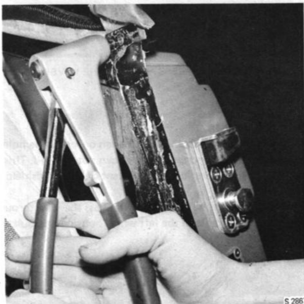
RIVETING WITH A POP RIVET TOOL
