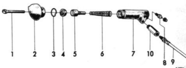
SLAVE CYLINDER, DISASSEMBLED
